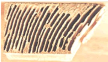
Western subterranean termites are highly destructive to Douglas fir and other common timbers used in the construction of a building. They can rapidly eat out the internal sections of structural timbers - devouring mainly the spring wood, and preferring to leave the harder summer wood sections.
